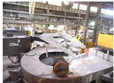
When the hoist is raised, it rises with the clamper open.
