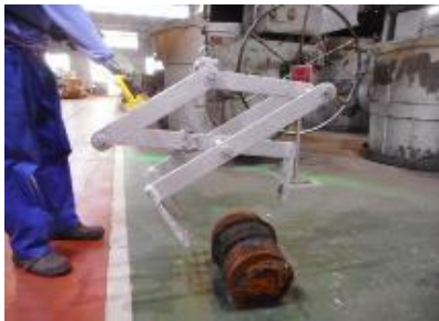
Align the clamper with the gate riser.
