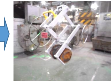
When the hoist is raised, the clamper closes and catches the gate riser.
