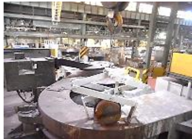
After moving, lowering the hoist opens the clamper and locks it.
